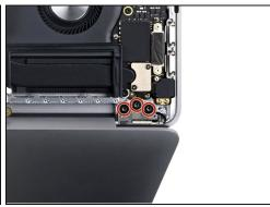
• Support the screen with one hand and use your free hand to remove the six T8 Torx screws securing the hinges.
