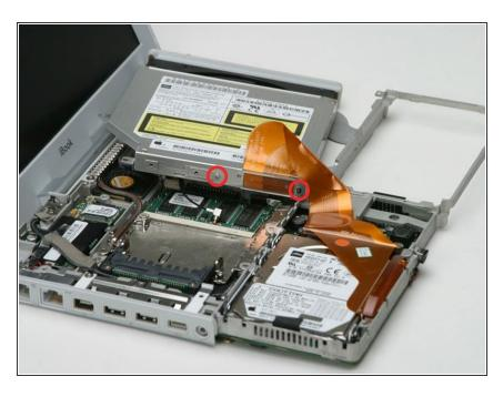
Remove the two 2.5 mm Phillips screws securing the large orange ribbon cable and thin metal bracket to the drive.
