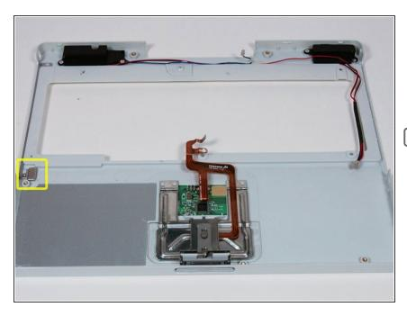
There is a magnet that allows the computer to detect when the laptop is closed. If this magnet is not present your computer will not automatically go to sleep. Be sure the magnet is in the position indicated.
