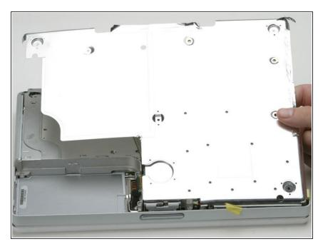
Lift the bottom shield off.
