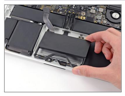
• Remove the SSD assembly from the upper case.
