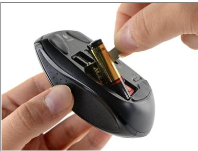
Pull the battery release tab away from the mouse until the two AA batteries come out.
