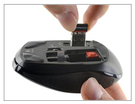
If the Nano Receiver is still in the mouse, push the bright orange button to remove it. It should pop right out.
