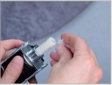
Your new pump may come with plugs on either end. Use an angled pick or small flathead screwdriver to pry these out before installation.
