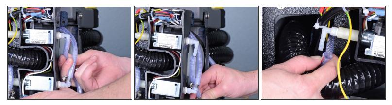
Pull the hoses at both ends of the pump straight off of their hose barbs to remove them.
