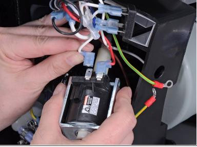
Pull the two connectors straight off of the pump to disconnect them from the pump.
