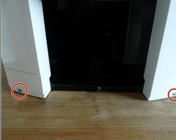
• Unscrew the two T10 Torx screws at the bottom of the front panel.
