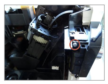
Unscrew the T15 Torx screw on the right.
