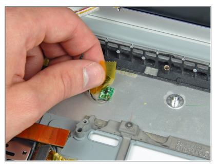
Peel back the piece of tape covering the left thermal sensor.
