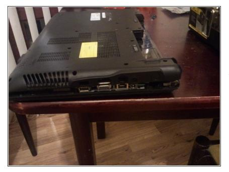
Unsnap case , it is best to start at the hinge joints. Work round the case towards the VGA port (RHS). The case needs to pop out over the port so ease the bottom out with your screwdriver. Work round towards the audio jacks (LHS). Lift the RHS of the case up and slide it towards the audio jacks to free them, as the casing cannot be eased over them.
