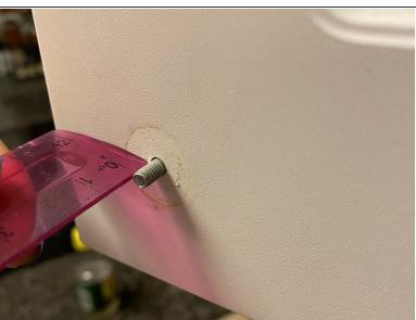
• If the screw looks too short, open the cabinet and see if the screw is all the way in. If not, screw it back in (then skip to step 4). If it is fully screwed into the cabinet and it is still too short (meaning you don't see at least 1/2 a centimeter of the screw), you will need a new screw.
