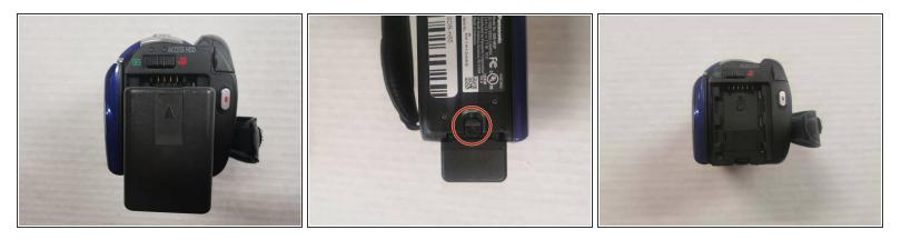
Gently slide the battery ejection button which is located underneath the battery and slide the battery out.
