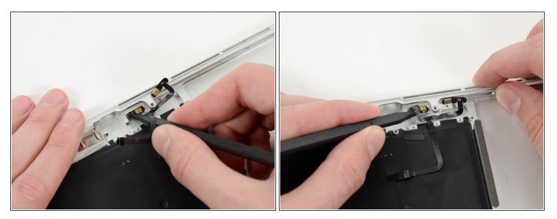
• Carefully pry the first microphone up off the upper case.
