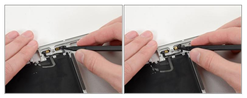
Gently wedge the tip of a spudger underneath the second microphone and push inwards to loosen the adhesive.
