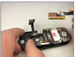
• Once the back casing is removed, disconnect the battery cable and remove the battery from the device.
