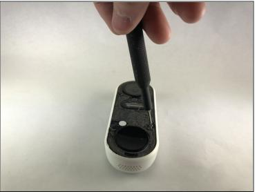
Peel back the cover stickers and use the Phillips #000 screwdriver to remove the four screws.
