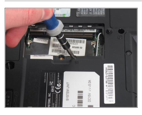
Use the Phillips #00 screwdriver to remove the 6.50mm screw holding the gray metal bracket in place.
