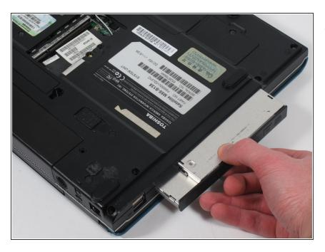
Pull the optical drive out of the laptop using your fingers.
