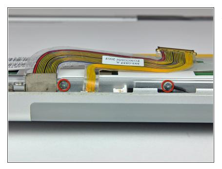
Remove the two Phillips screws securing the ground straps for the display data cable and LED driver board cable to the clutch cover.
