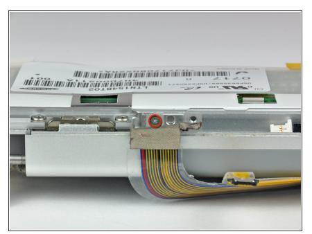
• Remove the Phillips screw hidden behind the display data cable.
