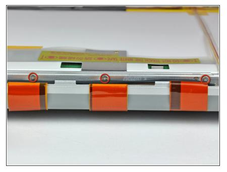
Remove the three Phillips screws behind antenna straps along the bottom edge of the display.
