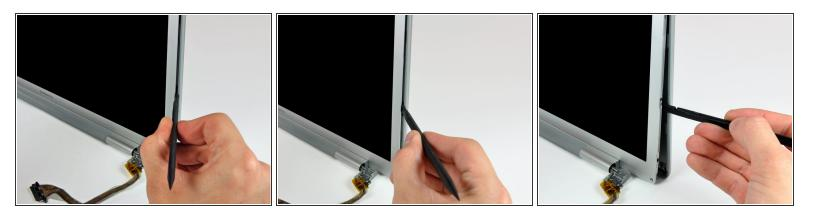
• Now that the right and bottom edges of the rear bezel are slightly separated from the front bezel, use a spudger to pop the rear bezel off the tabs near the lower right corner of the display.
