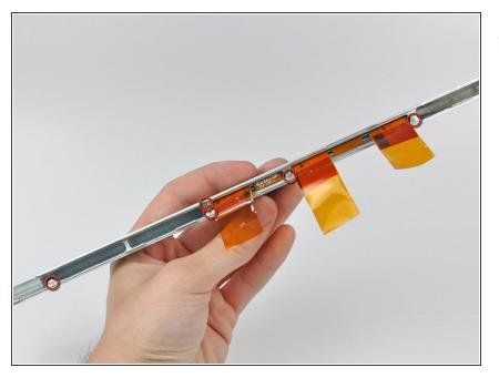
Remove the five small Phillips screws securing the plastic antenna cover to the inside of the clutch cover.
