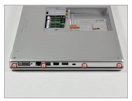
Remove the four 3.2 mm PH00 Phillips screws on the port side of the computer.
