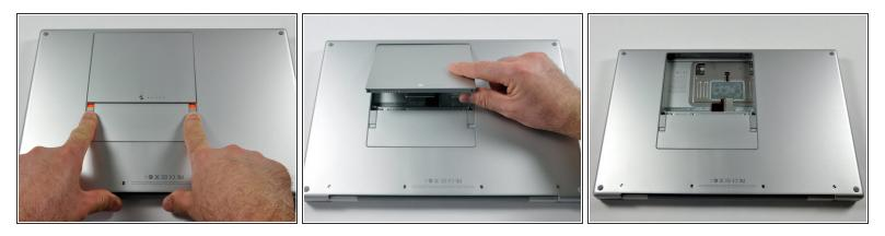
Use your fingers to push both battery release tabs away from the battery, and lift the battery out of the computer.
