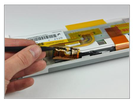
• Use the tip of a spudger to lift the LED driver board out of the clutch cover.
