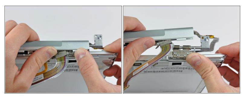
• Push the clutch assembly off each of the clutch hinges and remove it from the display.
