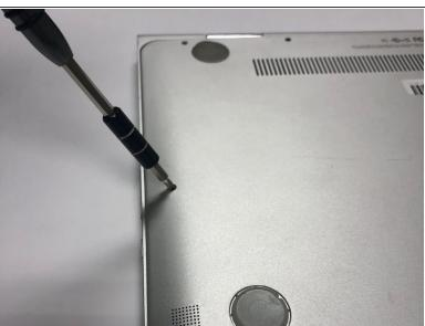
Using the Torx T5 screwdriver, remove the eight 8 mm screws on the bottom case of the laptop.
