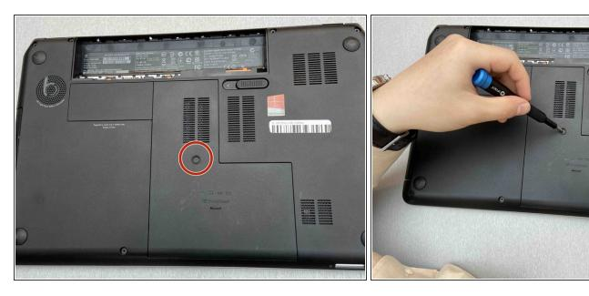
Remove the center screw using a Phillips #1 screwdriver.
