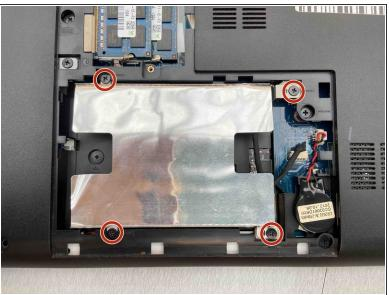
Remove the four Phillips #1 screws from the hard drive bracket.
