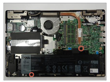
Use a Phillips screwdriver to remove the two 3 mm screws securing the battery to the laptop.
