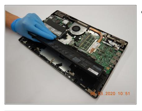
• Remove the battery up and out of the computer.
