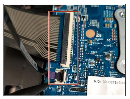
Disconnect the two ribbon cables connected to the motherboard by using the pointed end of a spudger to lift the plastic connector lids to allow the ribbon cables to be gently removed by hand.
