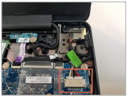
Disconnect the charging port cable from the motherboard using your finger or a spudger and gently pull it off.
