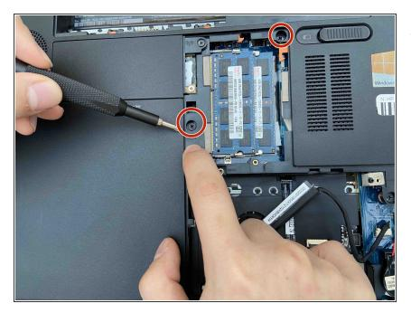
Remove the two screws that secure the keyboard to the laptop using a Phillips #1 screwdriver.
