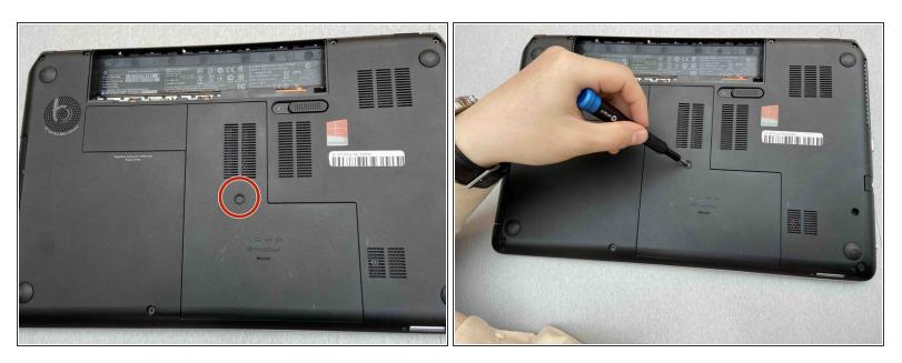
Remove the center screw using a Phillips #1 screwdriver.
