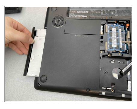
Pull the optical drive out of the base of the laptop. To reassemble your device, follow these instructions in reverse order.
