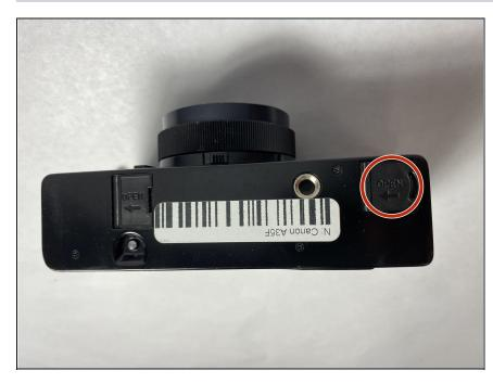
• Use your fingernail (or a iFixit opening tool), and push in the direction of the arrow to open the right compartment.
