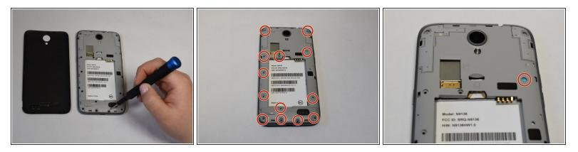
Use a Phillips #00 screwdriver to unscrew all 12 of the 3 mm Phillips screws located along the edges of the device's back panel, as well as the blue 3mm Phillips screw labeled "ZTE" located towards the top right.
