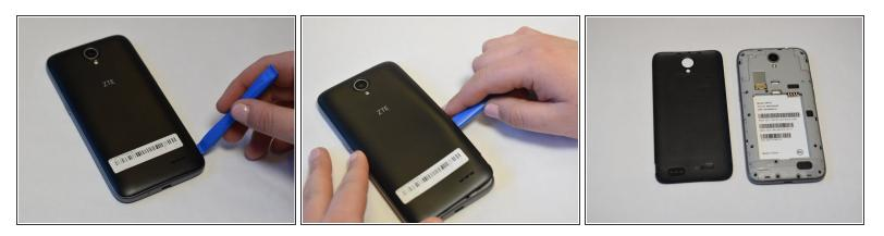
• Use the iFixit opening tool to open up the device by wedging the tool under the back case and popping it open.
