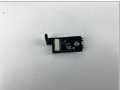
Disconnect the white connector from the sensor.
