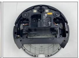
Push down on the black tab and remove the dust bin
