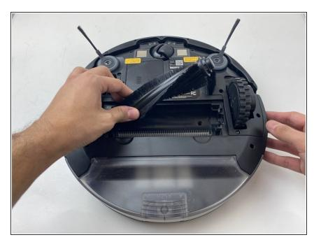
Pull the main brush slightly to the right to remove it from the compartment.
