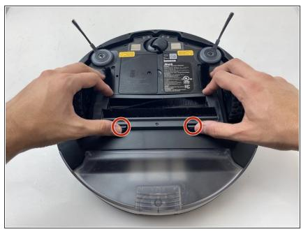
Push on the two tabs on the edge of the main brush cover and pull up to remove the cover.
