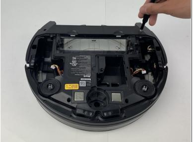
• Using a Torx TR15 screwdriver, remove the five screws from the bottom cover.
