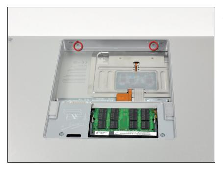
Remove the two 2.8 mm Phillips screws in the battery compartment near the latch.
