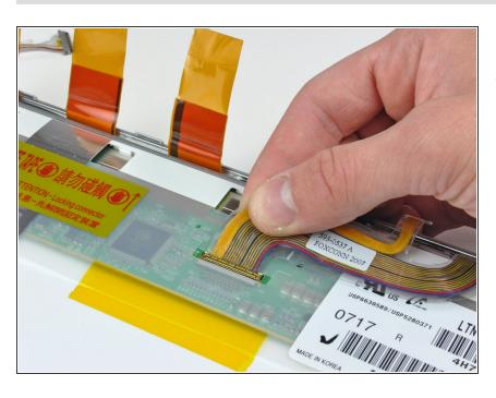
Disconnect the display data cable by pulling its connector toward the bottom edge of the display, away from the socket on the LCD.
