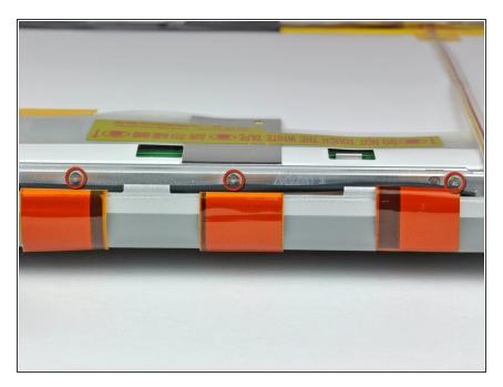
Remove the three Phillips screws behind antenna straps along the bottom edge of the display.
