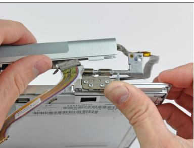
Push the clutch assembly off each of the clutch hinges and remove it from the display.
