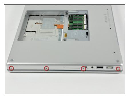
Rotate the computer 90 degrees again and remove the four 3.2 mm Phillips screws from the side of the computer.
