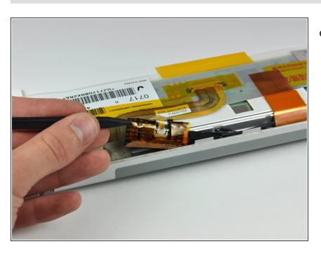
Use the tip of a spudger to lift the LED driver board out of the clutch cover.
