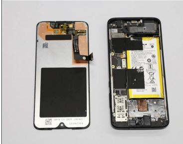
• Underneath this metal piece is the base of the cable. Use a spudger to vertically lift the connection out of its port.
