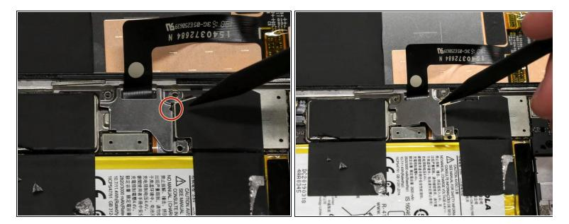
• Use the pointed end of the spudger to lift the metal casing where circled.
