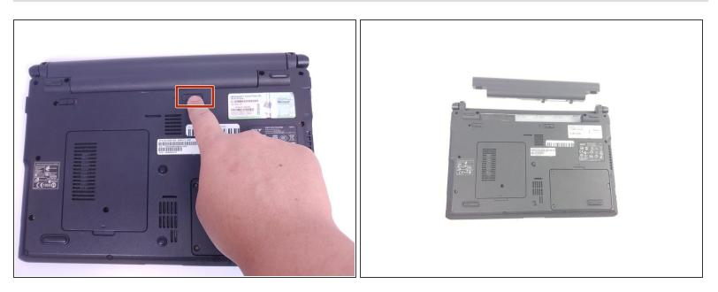
Slide the release button and remove the battery.
