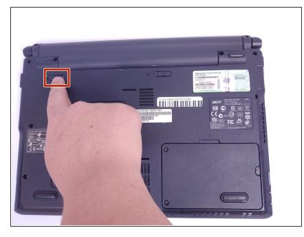
• Unlock the battery release by sliding it to the right.
