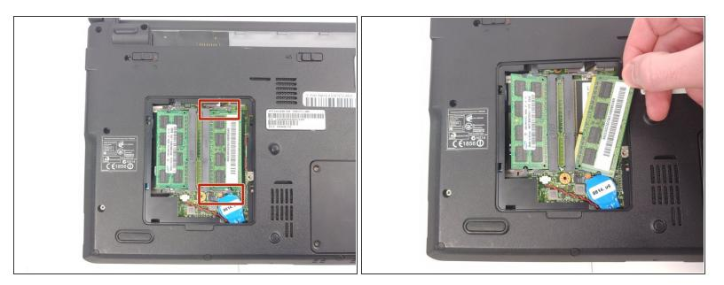
Push the side of the clips away from each other to release the RAM. Remove the RAM from the device.
