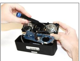
• Remove the 8mm Philips #0 screws holding speakers in place.
