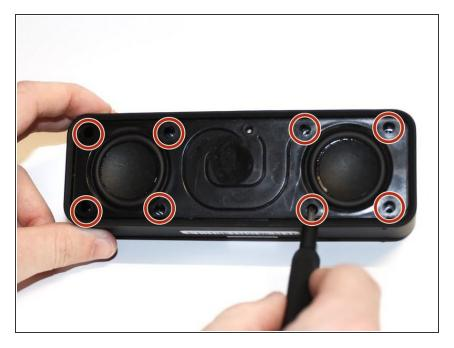
Remove the 10mm Philips #0 screws from speaker mount.
