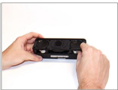
Use the metal spludger to pry off speaker mount.
