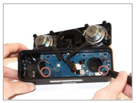
Remove the two 8mm Phillips #0 screws from the circuit board.
