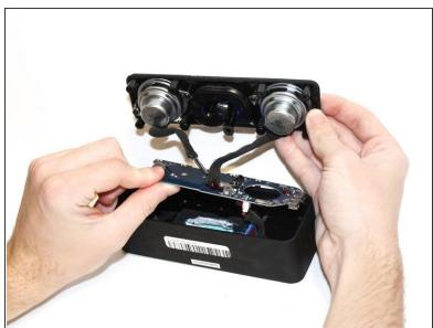
Carefully remove the circuit board from the speaker body.
