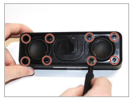
Remove the eight 10 mm Phillips #0 screws from the speaker mount.
