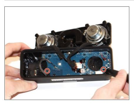
Use a Phillips #0 screwdriver to remove two 8mm screws from circuit board.
