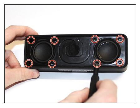
Use a Phillips #0 screwdriver to remove the eight 10mm screws securing the speaker mount to the speaker body.
