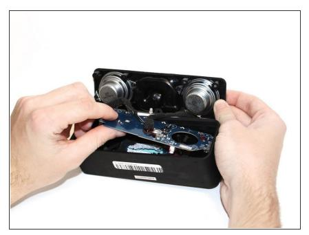
Carefully remove the circuit board from the speaker body.
