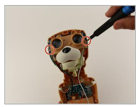
Using a Phillips #1 screwdriver, remove the two 12.5mm screws connecting the eyes to the rest of the mechanism.
