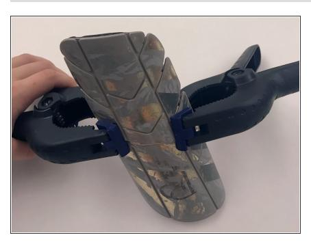
Align the clamps so that there are no spaces throughout the crack.
