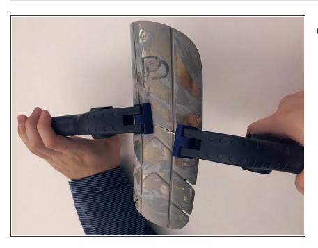
Put one clamp on either side of the crack.
