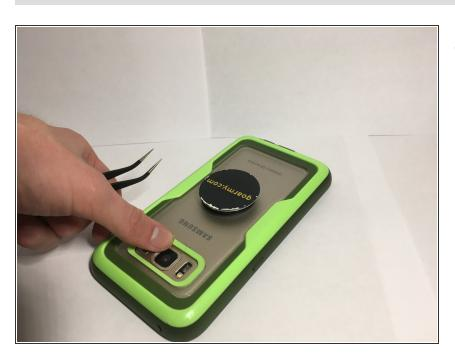
Press gently on the perimeter of the glass to ensure a strong bond between the glass and the phone, but not pressing hard enough to break the glass.
