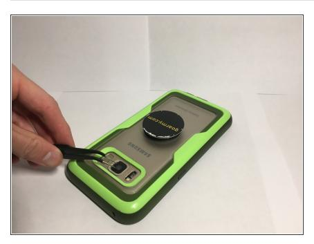
Center the new glass over the camera lens and lower it to the phone, careful to not scratch the exposed camera lens.
