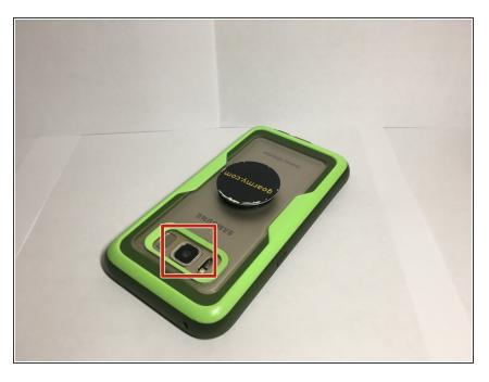
Check the surface for any residue or broken glass from previous cover.
