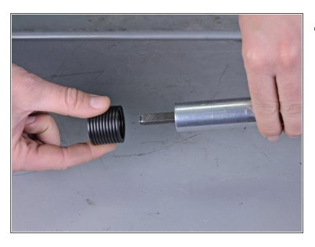
Slide the flexible tube off of the handle pipe and remove it.
