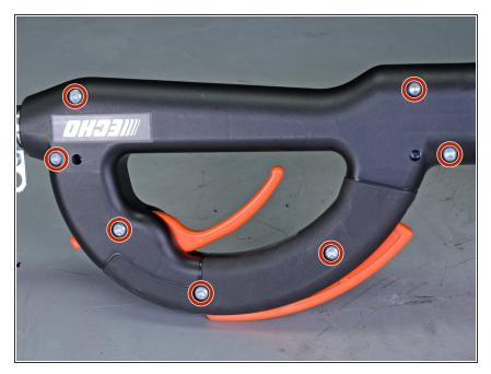
Use a T25 Torx screwdriver to remove the seven screws holding the control handle together.
