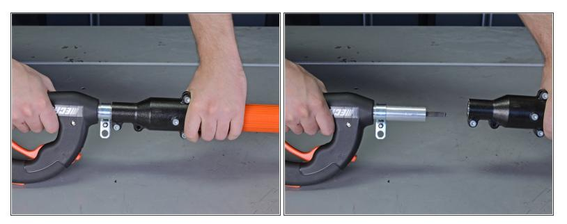
Remove the control handle from the main pipe assembly.
