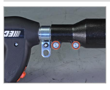
Use a T25 Torx screwdriver to loosen (but not remove) the two screws clamping the main pipe assembly to the control handle.
