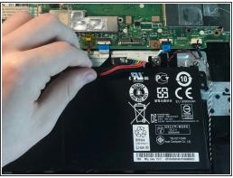
Gently and cautiously pinch the white ends of the battery connector cable and slowly pull it from the motherboard.
