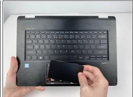
Gently remove the trackpad from the keyboard assembly by pushing out the trackpad lightly from behind.
