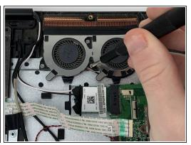
Using the Phillips #0 screwdriver, remove the eight 3 mm screws holding in the motherboard and the three 3 mm screws holding down the fan.
