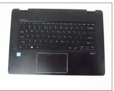
Remove the keyboard assembly by gently pulling it up.
