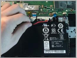
Gently and cautiously pinch the white ends of the battery connector cable and slowly pull it from the motherboard.
