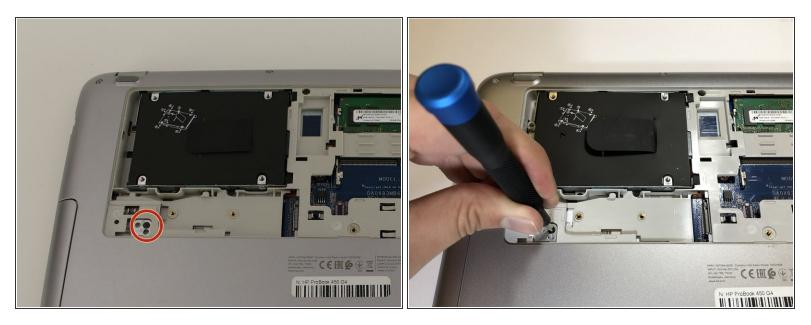
Use the Phillips #0 screwdriver to remove the black 3.2mm screw that secures the disk drive to the left side of the laptop.
