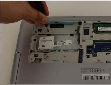
• Use a Phillips #0 screwdriver to remove the three 6.6mm screws from the upper left corner of the laptop.
