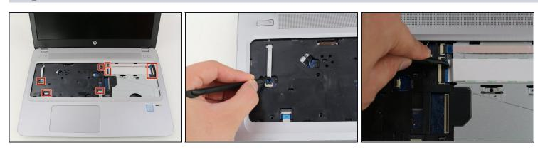
• Use the spudger to disconnect the nine cable connectors that secure the top case of the laptop to the body of the laptop.
