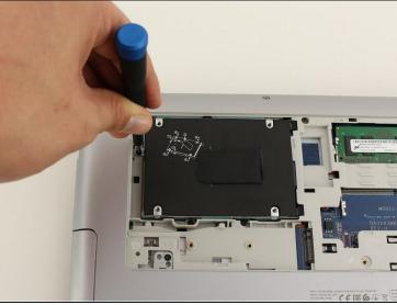
• Use the Phillips #0 screwdriver to remove the black 3.2mm screw that secures the hard drive to the left side of the laptop.
