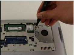
Use a Phillips #0 screwdriver to remove the two 6.6mm screws.
