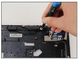
• Use the Phillips #0 Screwdriver to remove the two 3.5mm screws connecting the speakers to the top case of the laptop.
