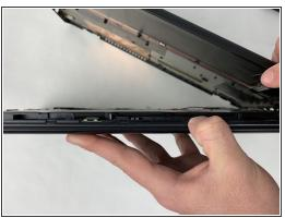
• Insert the Jimmy between the back cover of the laptop and the base of the laptop and then slowly use the Jimmy to pry off the back cover of the laptop.
