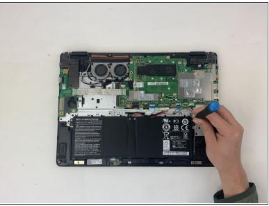
Use your Phillips #0 screwdriver to remove the two 3mm screws on the battery.
