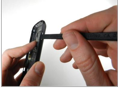
Holding the back case, gently push the power button in towards the center of the phone using a spudger.
