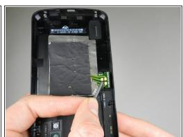
• To remove the volume button, push the button in towards the center of the phone using a spudger.
