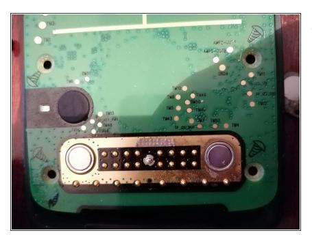
The PCB has exposed test pads for: I2S, JTAG, UART, Amp output, Power button and some pads named TM#
