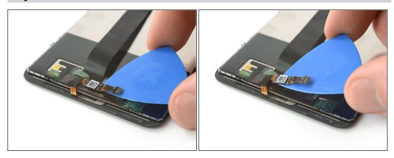
• Carefully slide an opening pick under the home button cable to loosen the adhesive underneath.
