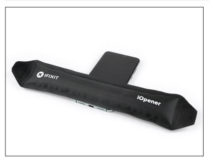
Apply a <u>heated iOpener</u> to the bottom end of the screen to loosen the adhesive underneath the loudspeaker. Apply the iOpener for at least two minutes.
