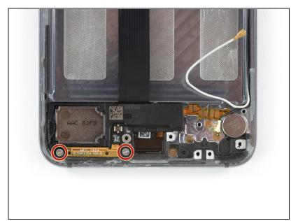
• Remove the two Phillips #00 screws (3.2 mm length).
