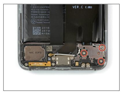
• Remove the three Phillips #00 screws (3.2 mm length).
