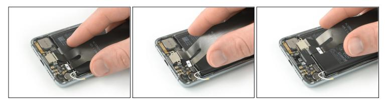
• Remove the charging port and main flex cable by lifting it upwards and then pulling it in the direction of the motherboard.
