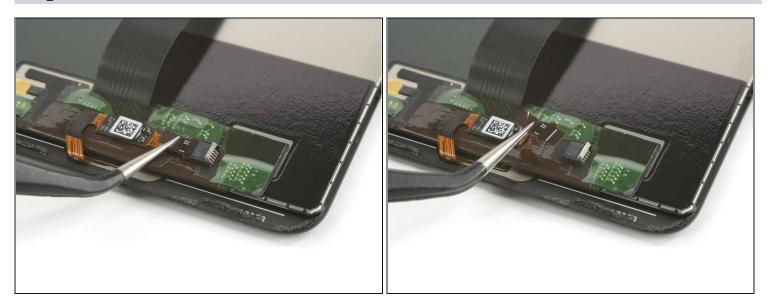
• Use a pair of tweezers to pull the home button flex cable out of its ZIF connector.
