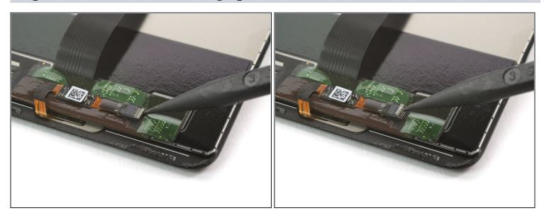
• Use the pointed end of a spudger to open the ZIF connector of the home button.
