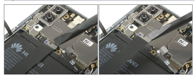
• Use a spudger to pry up and disconnect the display flex connector and fold the display cable out of your way to remove the battery.
