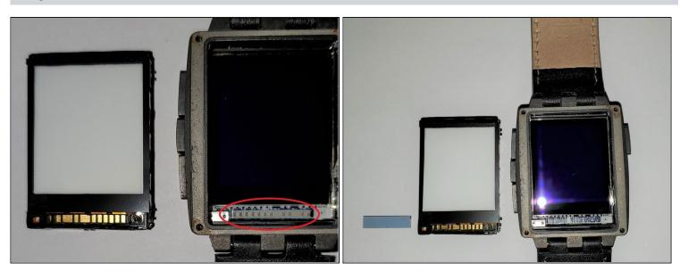
• The Zebra strip can stick to either the screen or the motherboard. Remove it with a pair of tweezers.
