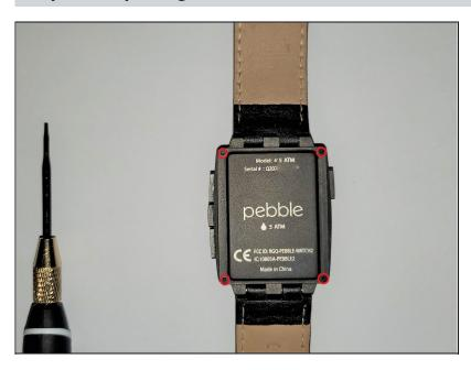
The Pebble Steel uses four Torx T3 screws to hold the rear of the watch housing on. First we'll remove all four screws.
