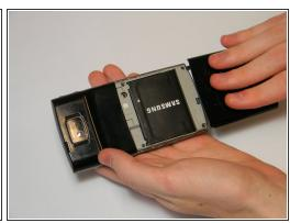
Apply downward pressure to the top of the battery panel while pulling down to slide it off the phone.
