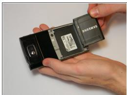
• Locate the grooves on the sides of the battery near the bottom of the phone. Use your fingers to pull the battery up and out of the phone.
