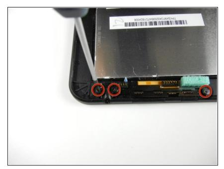
Unscrew the three 2.7mm Phillips #0 screws on the left and right sides of the headphone input.
