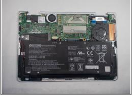
• Use a Torx #5 screwdriver to remove the six 3.5 mm screws holding the back cover to the laptop.
