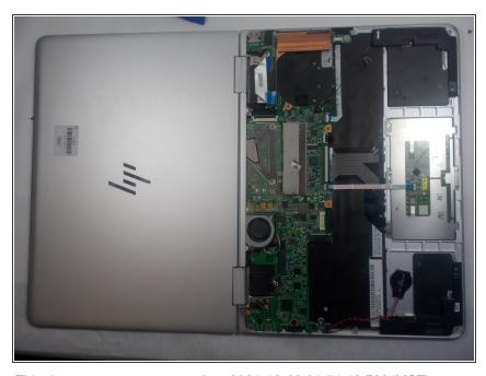
Lay the laptop flat on the table with the keyboard side facing the table and the motherboard facing up.
