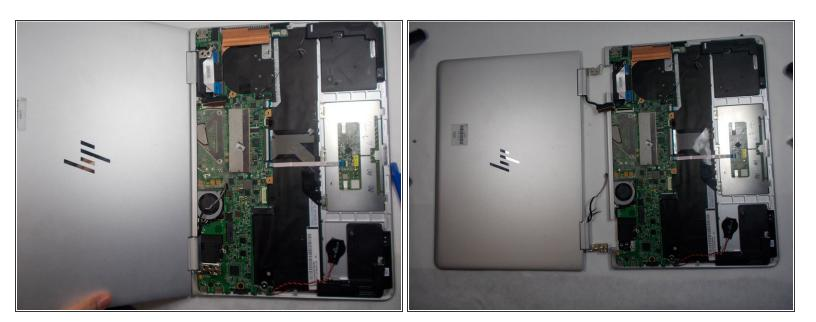
Separate the display from the bottom half of the computer(motherboard).
