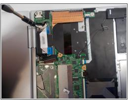
Using the Phillips #000 screwdriver, remove the four 1.0 mm screws that attach the display to the main body of the computer.
