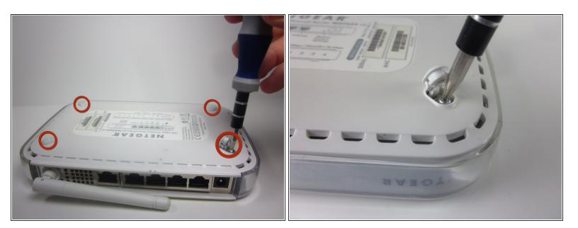
Unscrew the 4 11.8 mm T-8 Torx screws from each corner of the device.
