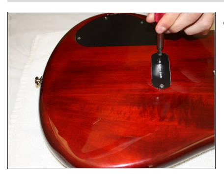
Use a Phillips #2 head screwdriver to unscrew both screws. Two #1 1mm long screws.
