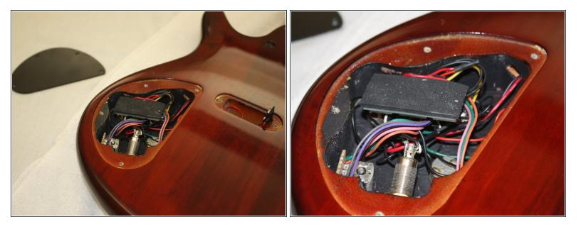
Remove the cap by lifting upwards, revealing the circuitry of the instrument.
