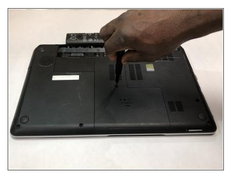
Using a Phillips #1 screwdriver, remove the 8.6 mm screw.
