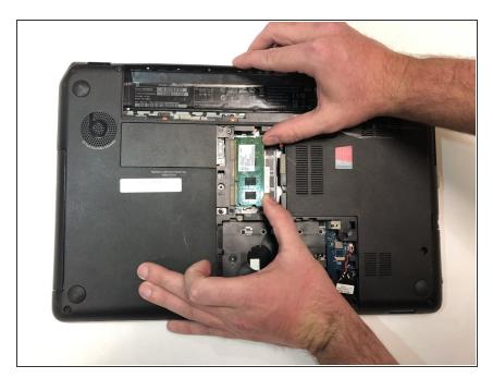
Lift gently up on the RAM to position it for removal.
