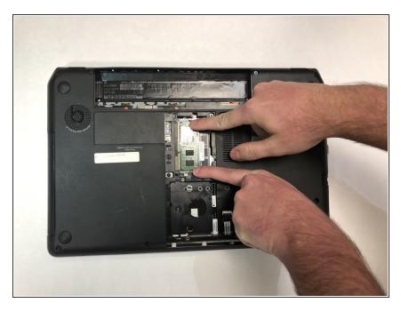
To release the RAM push out on the two release mechanisms holding it down.
