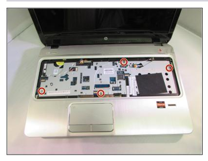
• Using a Phillips #1, remove the four 5.6mm silver screws.
