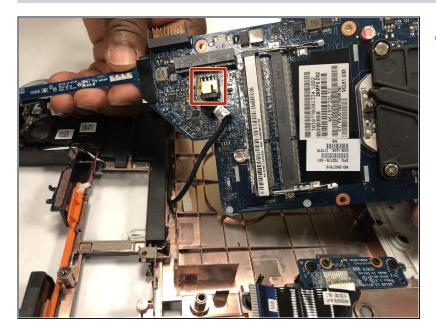
Pull the motherboard out of the laptop, taking care to detach the cable on the underside as you do so.
