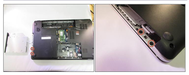
• Using a Phillips #1, remove the two 2.4mm screws.
